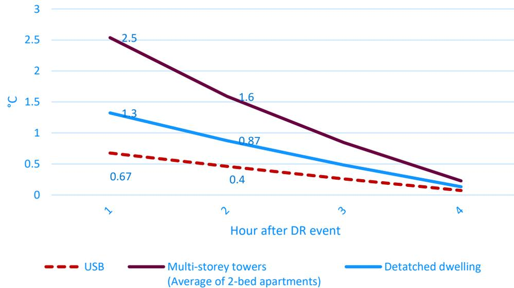
Cooling rate post electrified heating being switch-off
